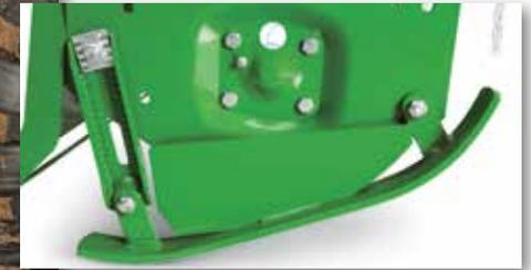
Working depth can be adjusted by the height of the skids, which is easily done with the adjustment bracket.
