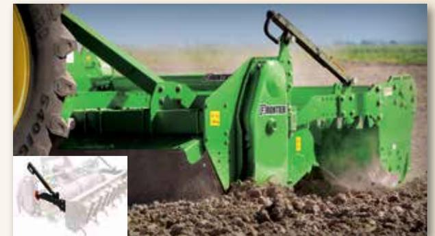
On the RT22 and RT23 Series, roller adjustment is easy using the two mechanical jacks placed on the sides of the rollers. Use a lower setting for more firming action, ideal for controlling wind erosion.
