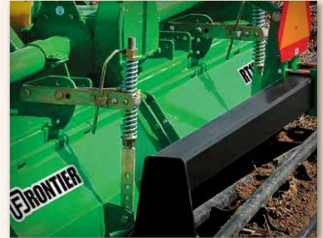
On the RT22 and RT23 Series, double springs provide consistent down pressure on the tailgate to level the tilled soil. Adjusting the height of the tailgate is easy: just remove the bolts and raise the tailgate to one of five settings. Use the low setting for a more level finish.
