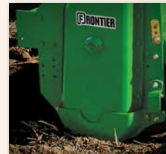
Heavy-duty wear shields on the RT23 Series help protect the gearcase from abrasion and premature wear.
