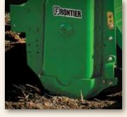
Heavy-duty wear shields on the RT23 Series help protect the gearcase from abrasion and premature wear.
