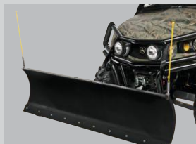
Standard Straight Blade, 66" Quick-attaching front blades have replaceable cutting edges, skid shoes, power lift and three-position angling.
