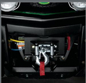
Warn@ Winch 3,500 lb. (1361 kg) winch. Includes a water-resistant remote control.
