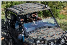
OPS Poly Roof All-year-round weather protection. Molded water troughs. Black or Camo.
