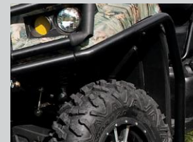
Front Fender Guards Protects front and side molding with heavy duty 2" steel tubing.
