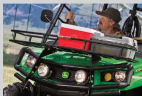
Front hood rack Generously sized rack (48" long, 13.5" wide by 3.5" deep) will carry up to 100 lb. of gear.
